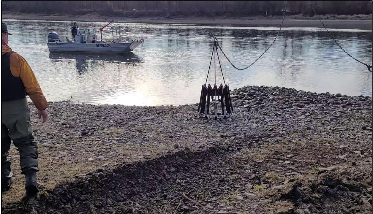
Photo 1.1 Tube screen initially tested as a substrate cleaning device on the Lower Patch on October 29-30, 2024; device is intended to be dragged on its side.
