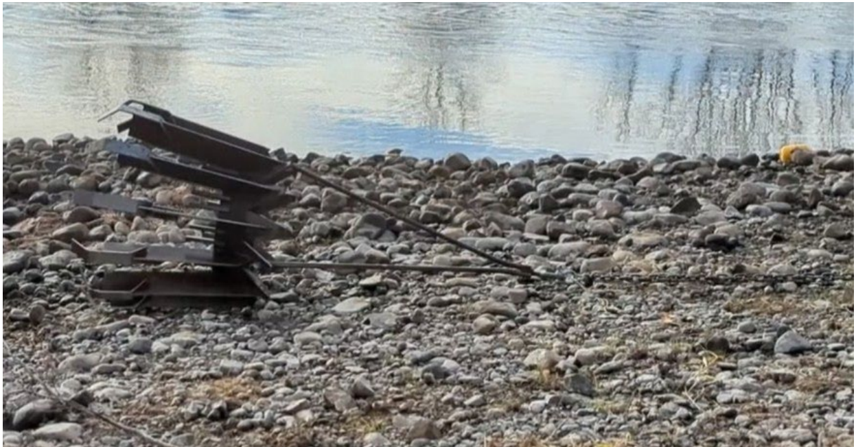
Figure 2. Tubescreen substrate sorting tool on the bank of the Nechako River at the Lower Patch white sturgeon spawning site.
