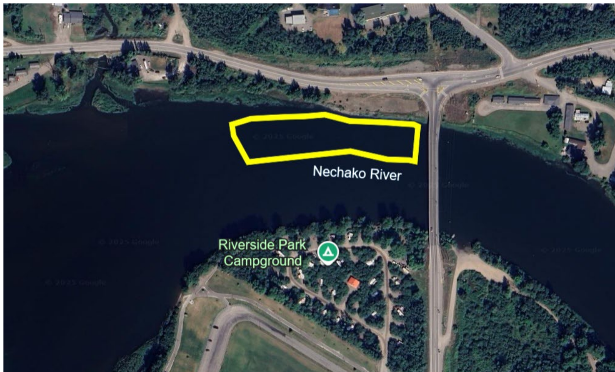
Figure 1. The Lower Patch restoration site in the Nechako white sturgeon core spawning area. The yellow polygon denotes the 40 m x 200 m gravel and cobble pad installed in 2011.
