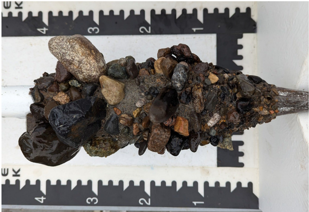
Figure 3. Freeze core sample of the ambient substrate in the Lower Patch restoration site before testing of the tubescreen sediment sorting tool. The large gravel and cobble layer installed in 2011 has persisted (left), but the interstitial spaces are infilled with fine sediment.
