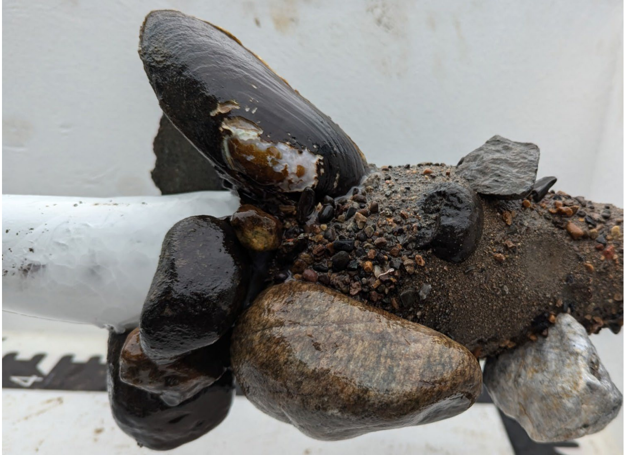
Figure 4. Freeze core sample of the substrate in the Lower Patch restoration site after testing the modified tubescreen sediment sorting tool. The large gravel and cobble have been raised to the bed surface and the fine gravel and sand have been deposited deeper into the bed. The ice frozen to the pipe (left) indicates that large substrate was present at the surface but did not adhere to the pipe.
