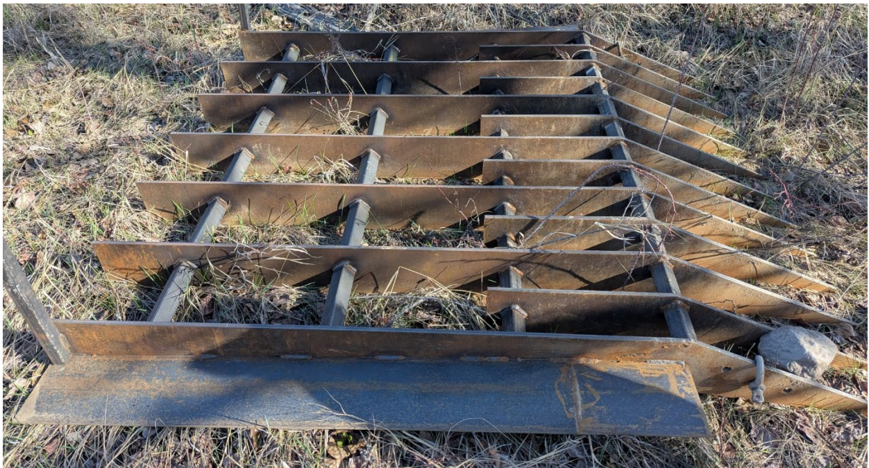
Figure 6. The 'sled' substrate sorting tool on land at the Lower Patch restoration site, April 2025.
