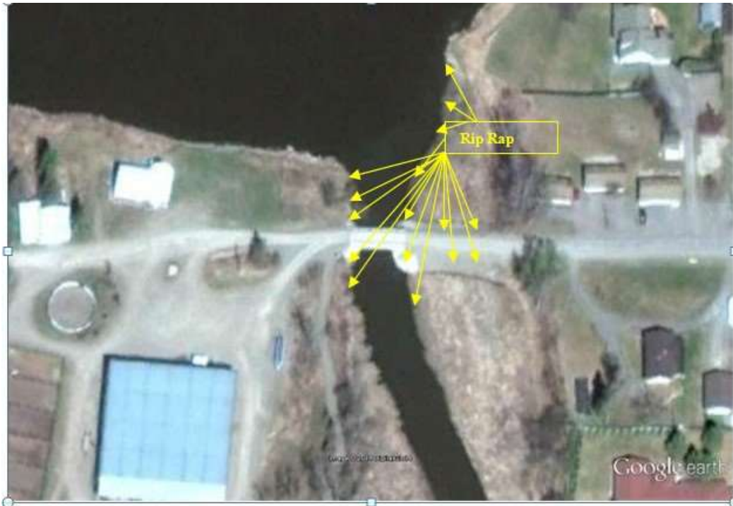
Figure 10. Proposed riprap locations for erosion control.
