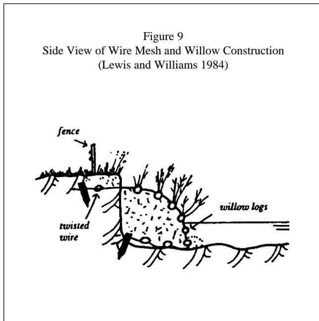
re-establishment of plants, as well as protecting recently planted vegetation. Live siltation barriers are effective immediately upon placement and protection increases as vegetation in the barrier becomes established. Live siltation resists high flows and is inexpensive to construct, usually 1/50 to 1/100 the cost of conventional engineered structures such as dykes and jetties (Schiechl 1980).
