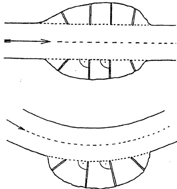
a bank. Construction of these barriers is labour intensive, and limited to a period when parent stocks for branch cuttings are dormant and water levels are low. Also, the need for a final rock layer requires that rocks be available, and their placement may require a backhoe or other heavy machinery.
