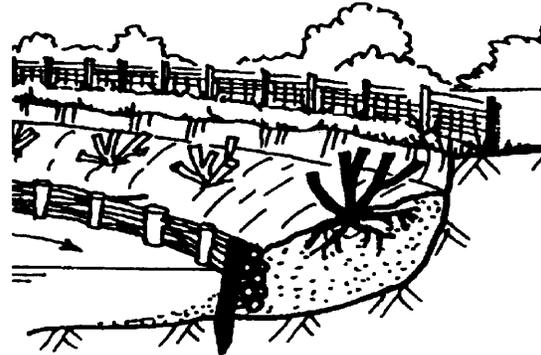
the integrity of the wire mesh is lost before vegetation can establish itself, the new bank may be subject to sudden failure.
