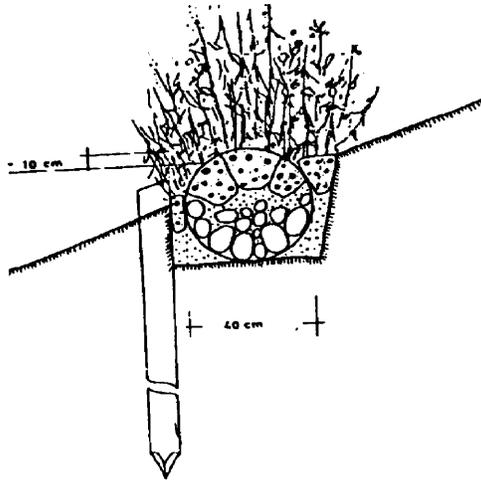
B. A variation of reed roll construction for fast water areas. A brush layer is placed underneath the reed roll.
