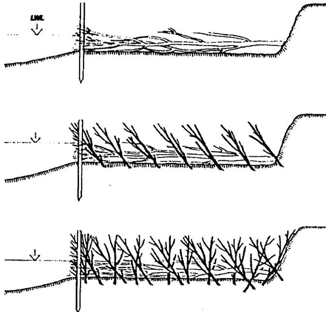
B. Repairing a break in the shoreline using a log brush barrier in conjunction with live siltation barriers and live brush (top view).
