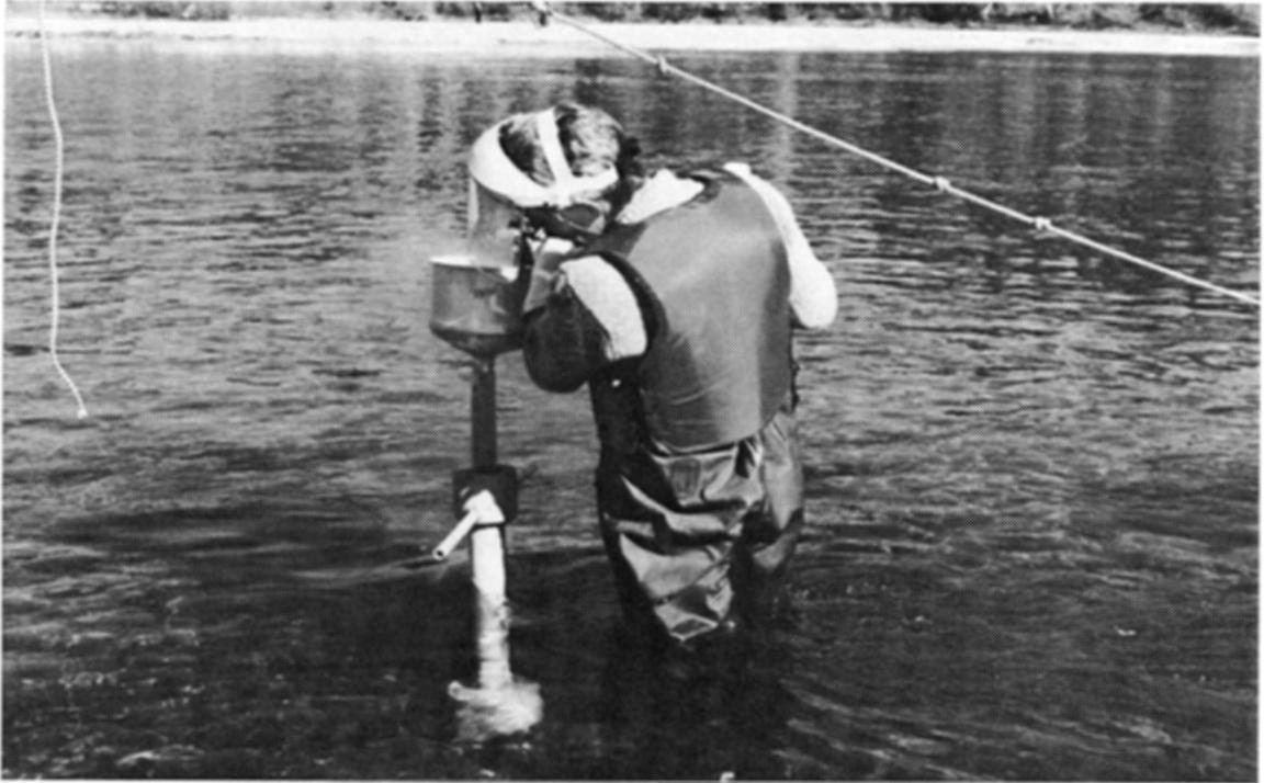
Plate 1 Core Barrel Inserted into Substrate (Note size of substrate).
