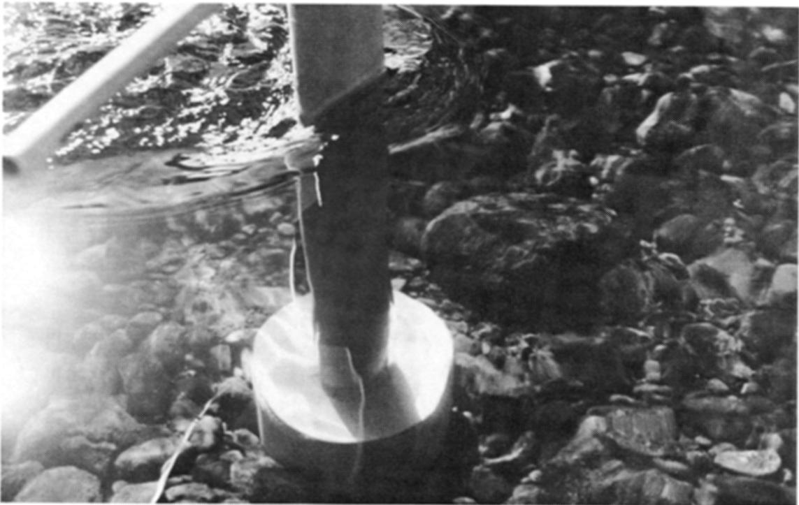
Plate 2 Adding Liquid Nitrogen to the Freeze-core Probe. (The probe projects approximately one foot above the top of the core barrel and handle).
