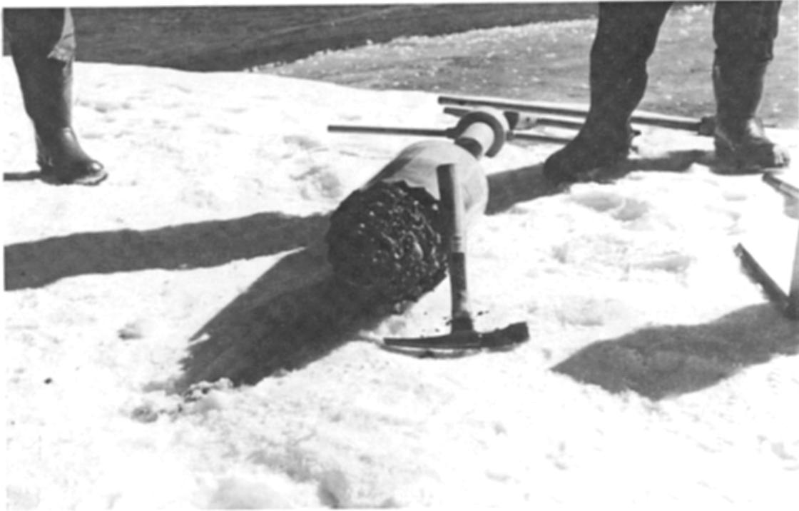
Plate 3 Core Barrel and Frozen Core
